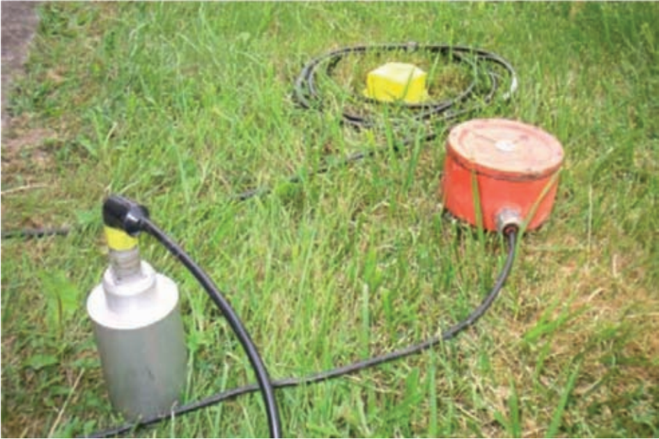
Fig. 1. The sensors we compared with different frequency peak: 1 Hz (left, grey, vertical component only), 4.5 Hz (right, orange, three-component) and 10 Hz (yellow, in the back, three-component).
