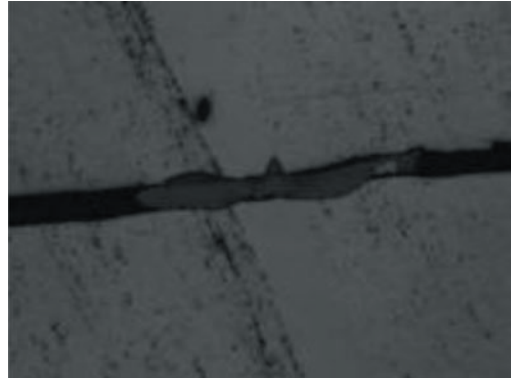
(b) Microscopic observation of coal sample bedding
