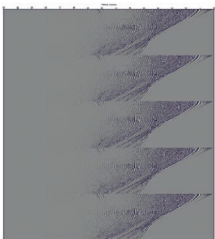
Fig. 8. A portion of real shot gathers as an example of real seismic data.
