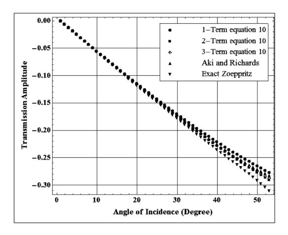
Fig. 2. (b) Plots of the  $T_{PS}$  coefficient.
