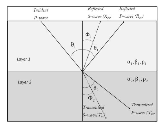
Fig. 1. Partitioning of the amplitude of a P-wave incident of an interface between two elastic solids.
