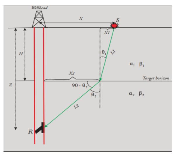
Fig. 3. Geometry of a VSP survey used to derive the offset-angle relationship and test the TAVO method.
