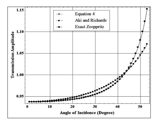
Fig. 2. (a) Plots of the  $T_{PP}$  coefficient.
