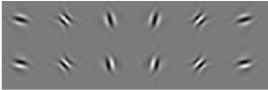
Fig. 1. The real (top) and the imaginary (bottom) part of the wavelet basis for the 2D complex dual-tree wavelet transform.
