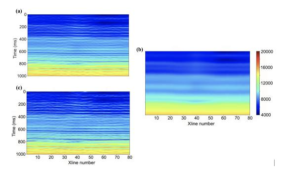
Fig. 8. (a) Actual, (b) initial, and (c) inverted AI models for inline #50.
