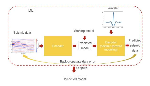
Fig. 1. Outline of the proposed CNN architecture for physics-based inversion. The acoustic impedance is estimated from stacked seismic gathers, and the obtained impedance model is used to generate seismic data by convolving the wavelet with the reflectivity series. Then the simulated data are compared with the observed data set.
