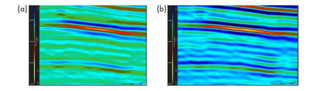
Fig. 10. Acoustic impedance predicted using (a) a homogeneous (constant AI) initial model and (b) the Hampson-Russell initial model.
