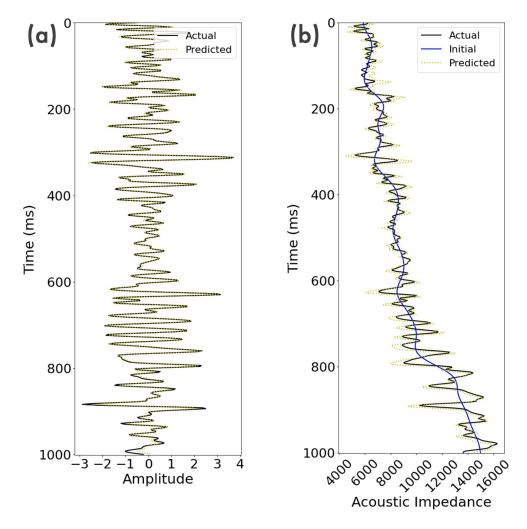
Fig. 7. (a) Comparison of the actual (black) and predicted (yellow) seismic traces for one of the CDPs. (b) Comparison of the actual (black), initial (blue), and predicted (yellow) acoustic impedance (AI) at the same CDP location
