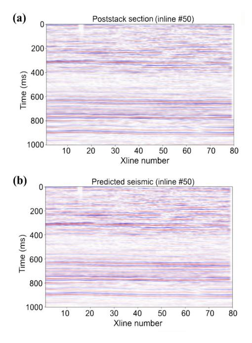
Fig. 6. (a) Inline #50 of the Hampson-Russell data set. (b) The mean poststack seismic data estimated by DLI.
