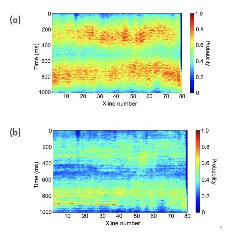
Fig. 9. Uncertainty maps of the posterior prediction of the acoustic impedance corresponding to the confidence interval between 30-70%: (a) Bayesian DLI; (b) Dropout DLI.
